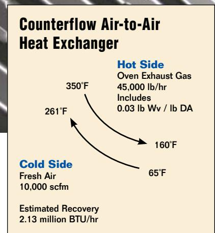
With a diagram of your proposed heat exchanger application, you can easily see what the duty is, and you can highlight important aspects or targets. You also could highlight pressure drops and static pressures as required.
